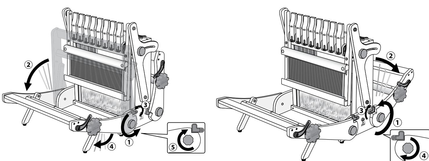
**Step 4:** Loosen knobs securing the beater supports, slide the beater completely forward and tighten the knobs.
