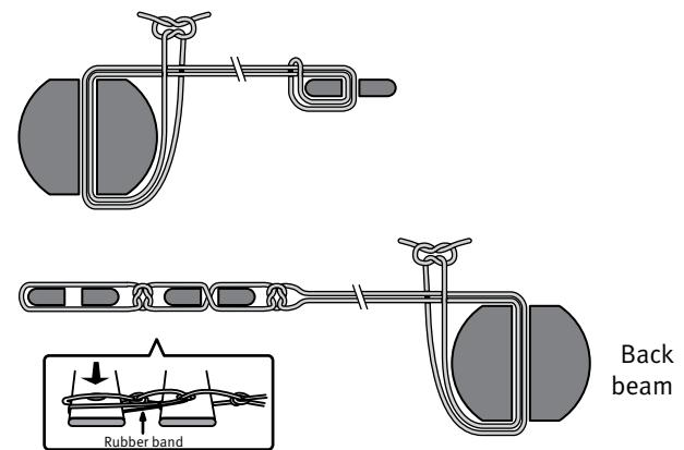
**Step 8:** To fold the loom, lift all the levers and reverse steps 4, 3, 2 and 1.
