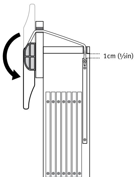
**Step 6:** Push the levers down and check the gap between the shafts and the castle top is approx. 1cm (1/2ins) on both sides. Adjust the height as necessary by moving the Texolv cord in the lever or on the screw head in the shaft end.
